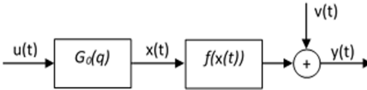
Figure 1.2: A Wiener system. G_d(q) is a linear dynamical system, f(x(t)) is a static nonlinearity and v(t) represents the measurement noise.
