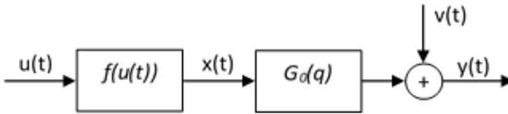
Figure 1.1: A Hammerstein system. G_0(q) is a linear dynamical system and f(u(t)) is a static nonlinearity and v(t) represents the measurement noise.
