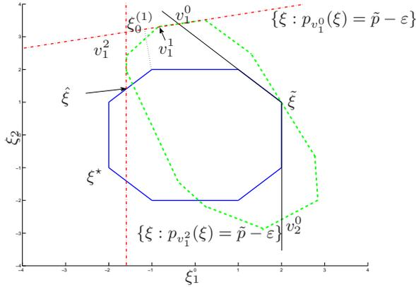
Figure 3: Hill detouring method. From a local optimum  $\tilde{\xi}$ , we can find  $v_1^0$ , which is the  $\gamma$ -extension along the active edge. Searching in the hyperplane of the level set, we arrive at  $v_1^1, v_1^2$ , and  $\hat{\xi}$ , successively.  $\hat{\xi}$  is feasible and has a less objective value than  $p(\tilde{\xi})$ , then we successfully escape from the local optimum  $\tilde{\xi}$ .
