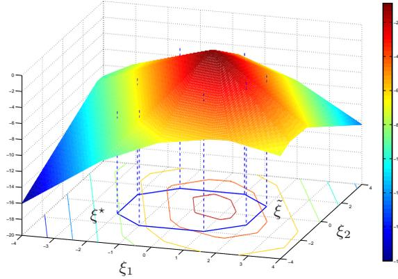
Figure 2: Plots of the objective function  $p(\xi)$  and the feasible domain  $A\xi \leq q$ , of which the boundary is shown by the blue solid line.  $\tilde{\xi} = [2, 1]$  is a local optimum and  $\tilde{p} = p(\tilde{\xi}) = -4.5$ ;  $\xi^* = [-2, -1]$  with  $p(\xi^*) = -8.2$  is the global optimum.
