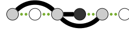
Fig. 3: Illustration of the column structure of the H_r matrix. Notice that the stencil is present in the structure of the Hankel matrix. The first, third, fourth and fifth row are linearly dependent. The linear relation is denoted by the black lines. The dotted line is the vectorized line of Fig. 2.
