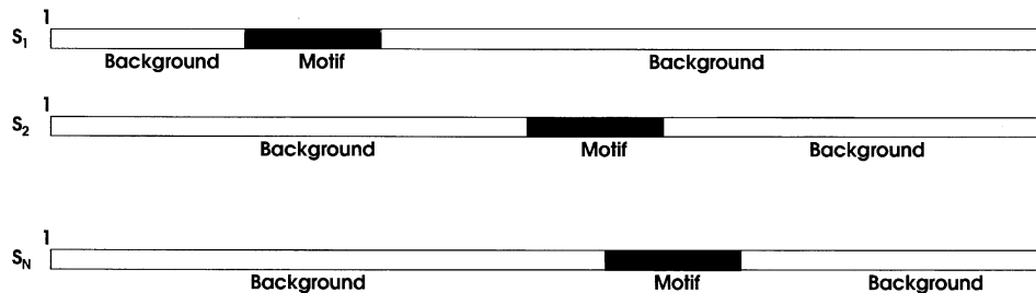
Fig. 8. In this basic sequence model, each sequence contains one and only one copy of the motif. The first part of the sequence is generated according to the background model \theta_0 , then the motif is generated by the motif matrix \theta_W , after which the rest of the sequence is again generated according to the background model.
