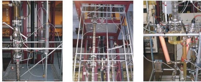
Figure 2: Pictures of the pilot-scale distillation column: condenser (left), packed section and feed introduction (center), and reboiler (right).
