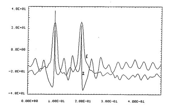
Figure 2: Results of Spectral Estimation. Real frequencies:  $f_1 = 0.1Hz$ ,  $f_2 = 0.2Hz$ . Curve 1: Spectral estimation by Periodogram. Curve 2: bý the proposed method.
