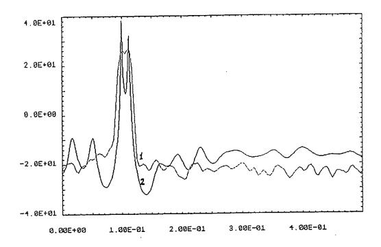
Figure 3: Results of Spectral Estimation. Real frequencies:  $f_1 = 0.1Hz$ ,  $f_2 = 0.11Hz$ . Curve 1: Spectral estiamtion by Periodogram. Curve 2: by the proposed method.
