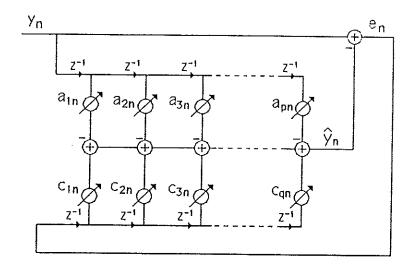
Figure 1: The Structure of an Adaptive IIR Filter
