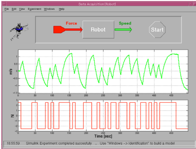
Figure 1: Data acquisition window. After the input is designed (bottom plot) it is applied to the process and the output is measured (top plot). The data is collected through file transfer (from DCS or PLC), from a Simulink model or from the RaPID real-time interface supporting sampling rates up to 40 kHz.
