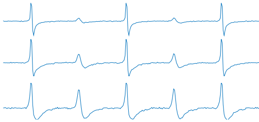
Fig. 16. Simulated outputs of a high-density microelectrode array for measuring neuronal activity using simulated spike trains as inputs.
