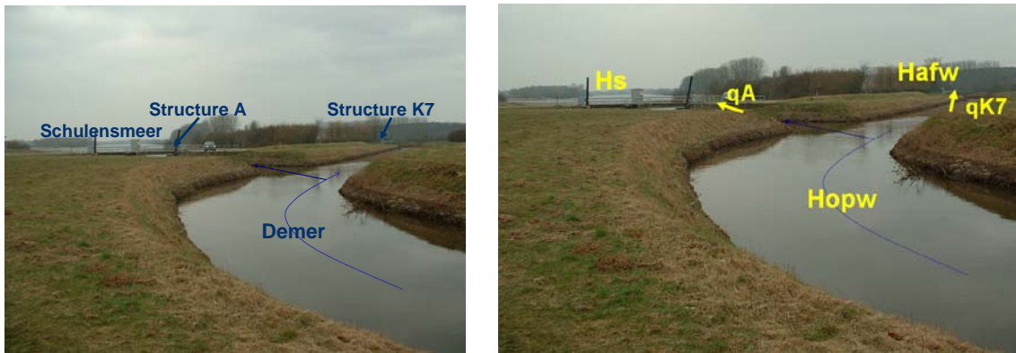
Figure 3: Photo of the river Demer and the “Schulensmeer” flood control reservoir in the background, together with the locations of the main water level and discharge variables
